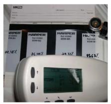
USING A SPECTRO-DENSITOMETER to measure opacity levels on site
